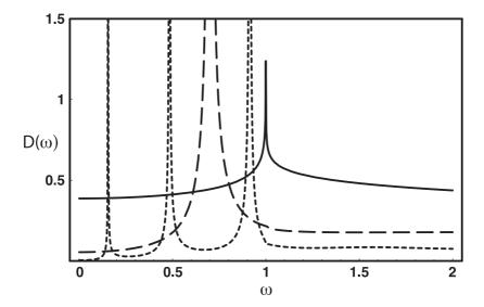
Figure 4:  $D(U_0, \omega)$  for the beam equation as a function of  $\omega$ ,  $0 \le \omega \le 2$ , for three different values of  $c_0$ :  $c_0 = 0.5$  (solid line),  $c_0 = 2$  (dashed line) and  $c_0 = 6$  (dotted line).
