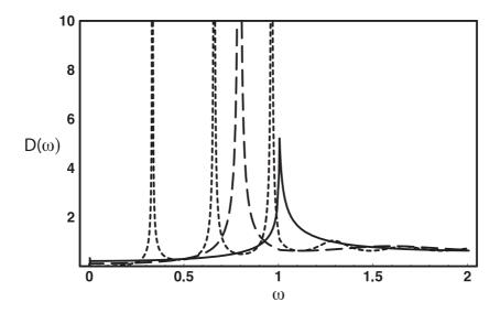
Figure 3:  $D(U_0, \omega)$  for the wave equation as a function of  $\omega$ ,  $0 \le \omega \le 2$ , for three different values of  $c_0$ :  $c_0 = 1.02$  (solid line),  $c_0 = 2$  (dashed line) and  $c_0 = 6$  (dotted line).
