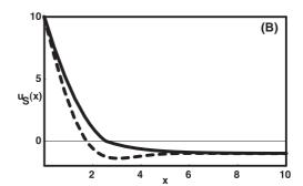
Figure 2: (A) The Touch-Down-Point  $c_0$  for the wave equation (solid line) and for the beam equation (dashed line) as a function of  $U_0$  for  $0 \le U_0 \le 100$  and (B) the static solution  $u_S(x)$ for the wave equation (solid line) and for the beam equation (dashed line) as a function of x,  $0 \le x \le 10$ , for  $U_0 = 10$ .
