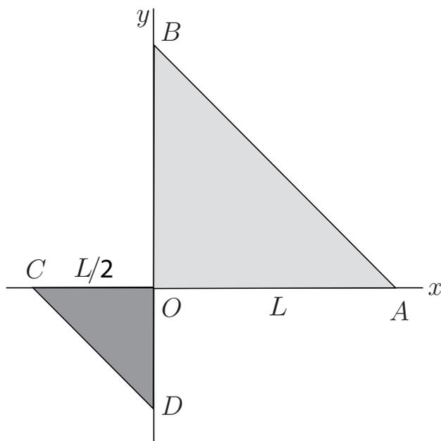
$$\underline{OAB} : I_{11} = I_{22} = \sigma \int_0^L dy \int_0^{L-y} y^2 dx$$
