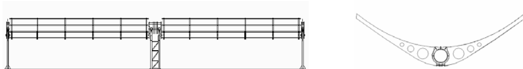
Figure 4: Sketch of the solar collector (portion), left, and sketch of a typical centering, right.
